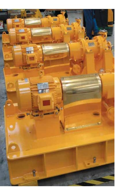
The HPGSP range comprises of pumps based on the HMD Kontro GS drive, built to API 685 specification, suitable for heavy-duty applications.
